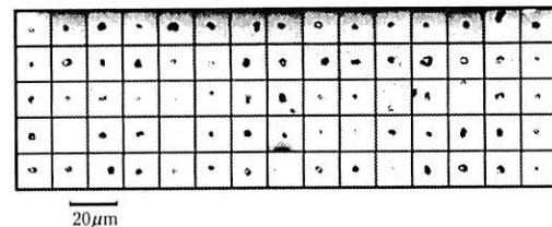
Fig.6 Observed images of agglomerates in class-6, prepared by dispersing WA # 6000 particles in 0.05wt.% sodium hexametaphosphate solution
